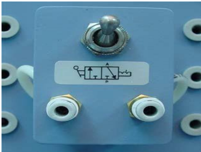
Fig. 10 (a) 3/2 directional control valve (b) Cross section
