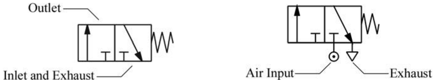
Fig 17 3/2 directional control valve (normally closed type)
