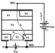
When the  $MT_2$  terminal is made positive with respect to the terminal  $MT_1$  and when positive voltage is applied at the gate terminal the path of the current flow from  $MT_2$  to  $MT_1$  will be  $P_1$ - $N_1$ - $P_2$ - $N_2$ . The junction between  $P_1N_1$  and  $P_2N_2$  are forward biased and junction between  $N_1P_2$  is reverse biased and breakdown occurs at this junction.
