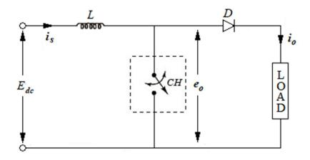
When the chopper is ON, the inductor L is connected to the supply and stores energy during on period  $T_{ON}$ . When the chopper is made OFF, the inductor stored energy as well as Source  $E_{DC}$  supply the load. Hence the load voltage becomes
