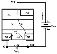
When the  $MT_2$  terminal is made positive with respect to the terminal  $MT_1$  and when negative voltage is applied at the gate terminal, initially the path of the current flow from  $MT_2$  to  $MT_1$  will be  $P_1-N_1-P_2-N_3$ . When the voltage applied at the  $MT_2$  terminal is further increased the junction  $P_2N_2$  is forward biased and the path of the current flow will be  $P_1-N_1-P_2-N_2$ . More Gate current is needed to turn the TRIAC.
