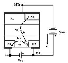
When the  $MT_2$  terminal is made negative with respect to the terminal  $MT_1$  and when negative voltage is applied at the gate terminal the path of the current flow from  $MT_2$  to  $MT_1$  will be  $P_2N_1P_1N_4$ .
