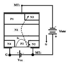
When the  $MT_2$  terminal is made positive with respect to the terminal  $MT_1$  and when negative voltage is applied at the gate terminal the path of the current flow from  $MT_2$  to  $MT_1$  will be  $P_2N_1P_1$ . The Junctions  $P_2N_1$  and  $P_1N_4$  are forward biased and the junction  $N_1P_1$  is reverse biased. So in this mode, TRIAC work in a negative biased region.
