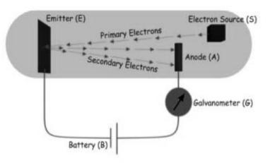
velocity striking electrons, transferred to the free electrons on the metal surface. Thus the free electrons may get sufficient kinetic energy to overcome the surface barrier and knocked out from the surface &start electron emission.
