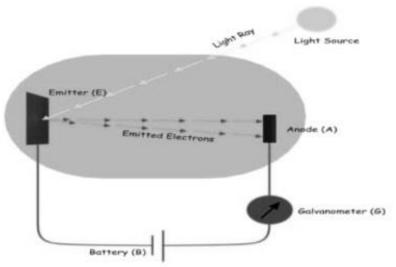
In this method, the energy of light falling upon the metal surface transferred to the free electrons within the metal to enable them to leave the surface. The greater theintensity (i.e. brightness) of light beam falling on the metal surface, the greater is the photo-electric emission.
