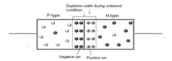
This pn junction does not allow flow of current. To make it suitable for electronics circuits we need to biasing (applying external voltage) pn-diode. There are two ways of biasing pn-diode (i) Forward biasing
