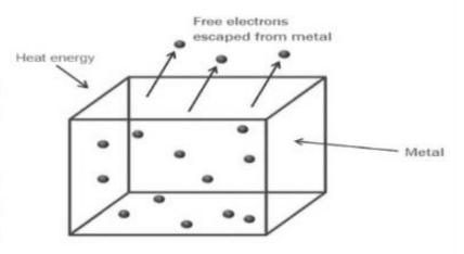
from one atom to another but can not leave the surface of the metal to provide electron emission.
