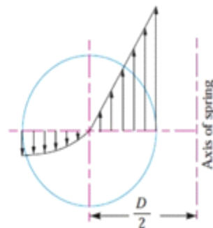
(d) Resultant torsional shear, direct shear and curvature shear stress diagram.
