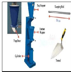
Fig. 2: Compaction Factor Apparatus with Allied Tools
