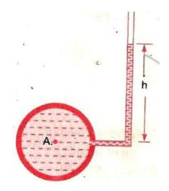
It is the simple form of manometer used for measuring gauge pressures. One end of this manometer is connected to the point where pressure is to be measured and other end is open to the atmosphere as shown in Figure. The rise of liquid gives the pressure head at that point A. Then pressure at A
