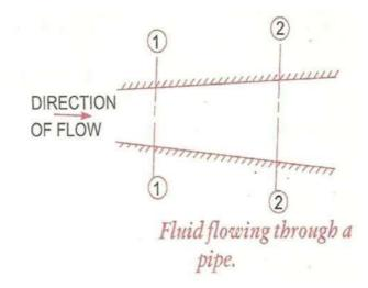
Let  $V_1$ = average velocity at cross-section 1-1.
