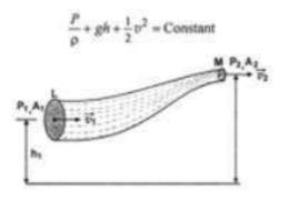
Proof: Let us consider the ideal liquid of density p flowing through the pipe LM of varying cross-section. Let P<sub>1</sub> and P<sub>2</sub> be the pressures at ends L and M and A<sub>1</sub> and A<sub>2</sub> be the areas of cross-sections at ends L and M respectively. Let the liquid enter with velocity V<sub>1</sub> and leave with velocity v<sub>2</sub>. Let A<sub>1</sub> > A<sub>2</sub>. By equation of continuity,
