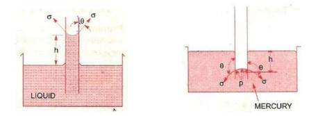
Its value depends upon the specific weight of the liquid, diameter of the tube and surface tension of the liquid.
