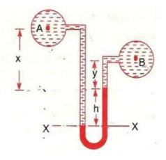
Let the two points A and B are at different level also contains liquids of different sp.gr. These points are connected to the U-tube differential manometer. Let the pressure at A and B are  $P_A$  and  $P_B$ .
