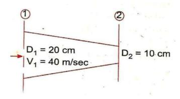
Solution. Given :  $D_1 = 20 \text{ cm} = 0.2 \text{ m}$   $\therefore \text{ Area,}$   $A_1 = \frac{\pi}{4} D_1^2 = \frac{\pi}{4} (.2)^2 = 0.0314 \text{ m}^2$   $V_1 = 4.0 \text{ m/s}$   $D_2 = 0.1 \text{ m}$  $A_2 = \frac{\pi}{4} (.1)^2 = .00785 \text{ m}^2$
