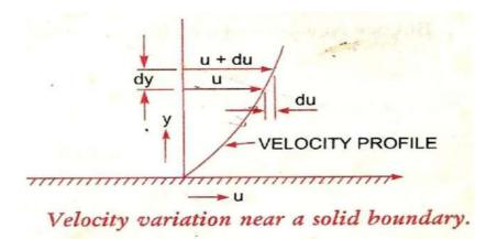
The viscosity together with the with the relative velocity between the two layers while causes a shear stress acting between the fluid layers, the top layer causes a shear stress on the adjacent lower layer while the lower layer causes a shear stress on the adjacent top layer.
