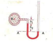
For measuring vacuum pressure, the level of the heavy liquid in the manometer will be as shown in figure. Then Pressure above A-A in the left column
