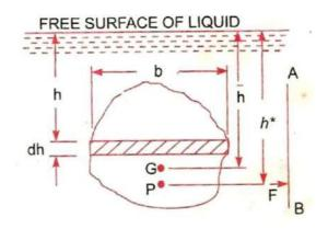
The resultant force F is acting at P, at a distance  $h^*$  from the free surface of liquid.
