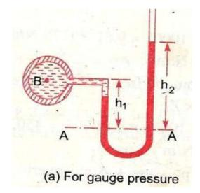
Pressure is same in a horizontal surface. Hence pressure above the horizontal datum surface line A-A in the left column and in the right column of U-tube manometer should be same pressure above A-A in the left column
