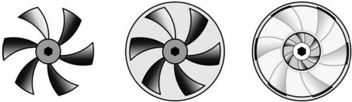
Figure 1. Impeller Types (l to r): Open, Semi-Enclosed (or Semi-Open), Enclosed.
