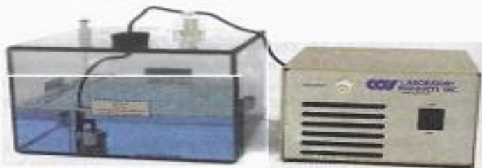
Ultrasonic humidification system.
