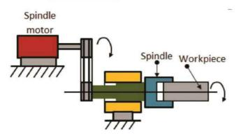
The spindle drives are used to provide angular motion to the workpiece or a cutting tool. These drives are essentially required to maintain the speed accurately within a power band which will enable machining of a variety of materials with variations in material hardness. The speed ranges can be from 10 to 20,000 rpm.
