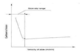
At the commencement of the movement, the coefficient of friction is very high, but as the velocity increases it falls rapidly and beyond a certain critical velocity it remains almost constant. Thus, to start motion/movement, the force to overcome friction has to be correspondingly high. This phenomenon is known as, stick-slip phenomenon.
